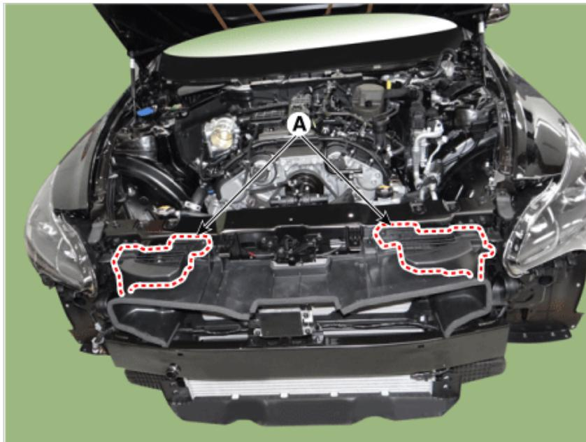
3. Remove the air guard (A) by loosening the bolts after separating the wiring fixing clip.
